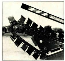
The Charles Machine Works ditch witch tough tooth 90 digging assembly
