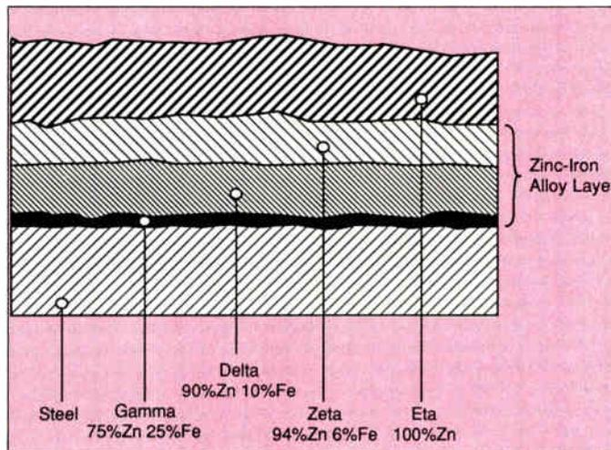
two ways. First, because of the metallurgical interlock of zinc, zinc-iron alloy and steel, an impervious coating is formed to shield the steel from corrosive elements. And second, the zinc and zinc-iron alloy layers furnish galvanic protection by sacrificing themselves ever so slowly when exposed to corrosive environment.
