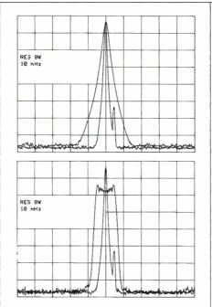
a) (above) Filter shape absorbing an adjacent signal
