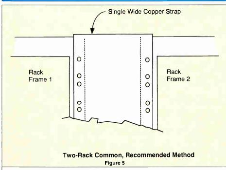
than 1/16-inch thick and which will still be effective even if only 10 mils (0.01-inch) or so in thickness. Larger pieces can be obtained from a metals merchant by asking for soft copper in rolls, alloy 110. Smaller amounts of thinner material can be conveniently
