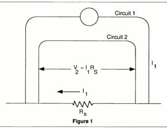
or 0.00006 inch. Since the intrinsic resistance of steel is eight times that of copper, at 6 MHz the net resistivity of steel is 135 times that of an identical piece of copper. A current flowing across one inch of steel will have the same voltage drop as it would flowing across over 11 feet of copper.
