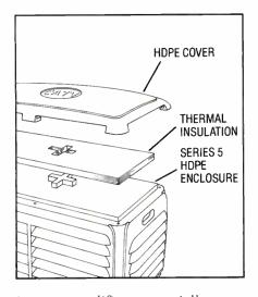
in your amplifiers, especially on the IC boards and power supplies. Independent field testing of "HDC" covers against competitive metal enclosures indicates this percentage could be even higher, depending upon the size of metal enclosure used in relationship to the amount of active and passive equipment spliced in it.
