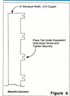
The way to bring these widely separated amplifiers together is to install a wide copper rack-to-rack connection from surface X to surface X as shown in Figure 4. This single copper cross piece will beat any pre-existing current return path by a wavelength and
