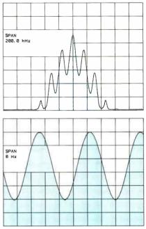
(a) (above) Measure modulation sidebands in a narrow frequency span
