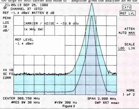
display range, compared to about 20 dB on an oscilloscope. Accurate amplitude measurements can be made in the first 70 dB below the reference level; however, the lowest 10 dB of the CRT range is useful for identifying low-level signals. The log amplifier changes its gain depending on the level of the input signal, compressing high-level signals so that high- and low-level signals can be displayed simultaneously, Figure 3.
