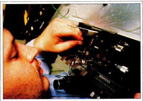
An engineer feeds optical fiber into a fusion splicer
