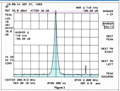
reference-level setting so that a signal at or below the reference level will not exceed mixer compression. You can change attenuation over a 60 dB range using a softkey; however, the analyzer does not allow a combination of refer-
