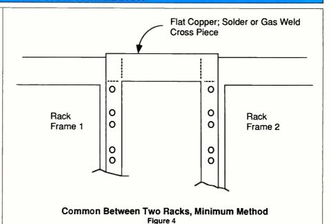
Assume that there is no electrical connection between rack frame and rack sheet metal.
