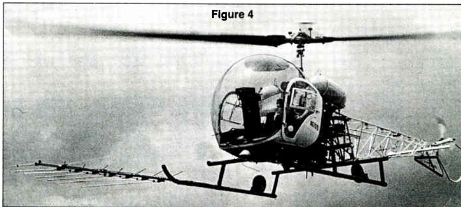
Multi-element antenna mast-mounted to helicopter
