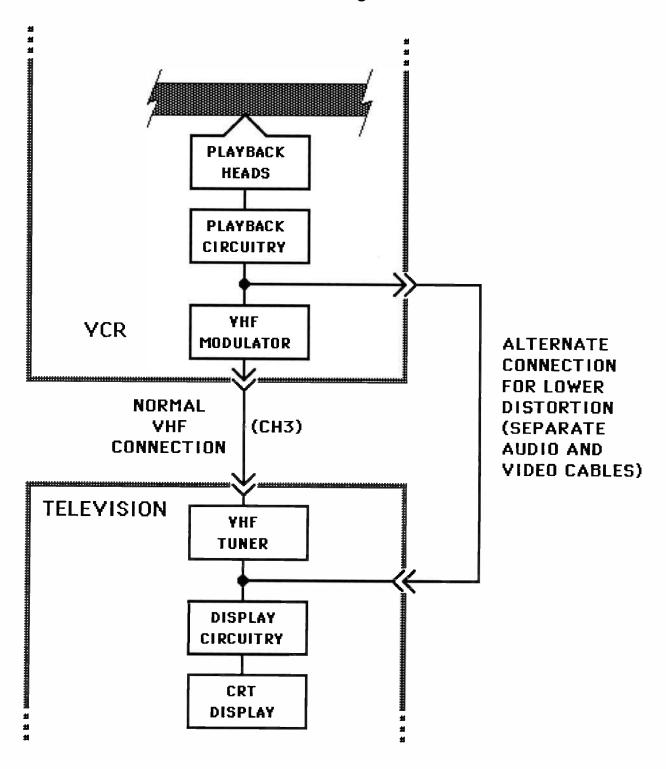
SIMPLIFIED YCR AND TY SIGNAL PROCESSING DIAGRAM
