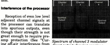
ing off-air interference from direct output showing spurious outputs into adjacent channels
