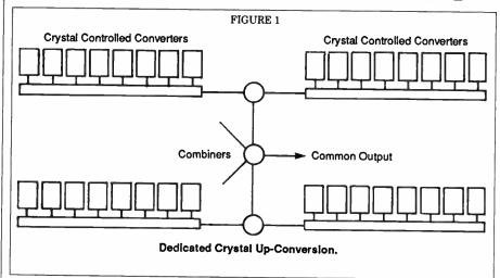
headend construction or channel addition are available today: non-modular (no front panel modules) frequency agile up-conversion (FAC); and front panel modular, dedicated crystal up-conversion (DCC).
