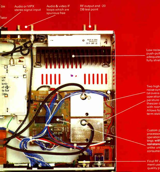
Low noise, hybrid power, push-pull amplifier that is adequately heatsinked and fully shielded.
