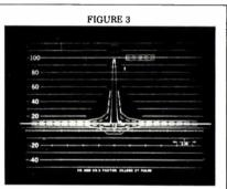
"Character Generator Pulse" - 75 Nanosec Wide -15 Nanoseconds Rise and Fall Times
