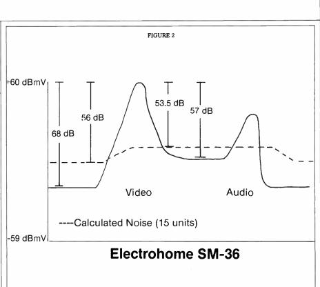
video signal-to-noise ratio provided by the satellite receivers to be high enough to provide noise-free video.
