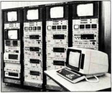
For accuracy, SMPTE time code is used to locate ad spots and programs on the tapes. A directory is written onto the beginning of each tape that uniquely identifies each spot or program and its location. Because of this, tape searching is reduced and the chances of playing the wrong spot are minimized.
