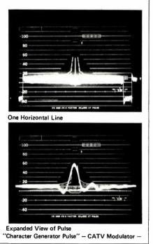
carefully controlled to produce an energy distribution vs. frequency which is approximately 6 dB down at 2 MHz and essentially zero above 4 MHz.
