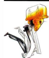
Our unique eight-point suspension and hinged drop chute with removable gate isolate vibration from the machine and cable. Service loops can be restrung without cutting or splicing. And only Case offers a front trencher, rear plow combination.
