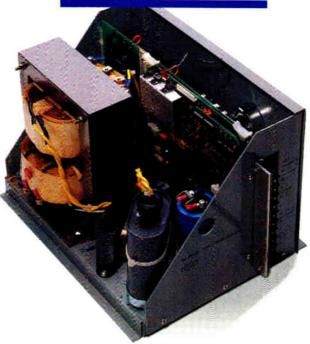
Pull off our cover and you'il see why Alpha is the CATV Standby Power Supply leader. Sure, we could have designed a system using two transformers like most manufacturers, but no, we decided that a single ferro-transformer would be more reliable. It was gutsy, it was innovative, and it works.
