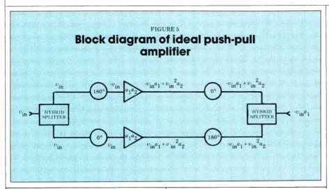
where 0.707 represents the voltage division of the 3 dB split. The phase inverter reverses the polarity of one signal. At the amplifier inputs 2 and 2', the signals are:
