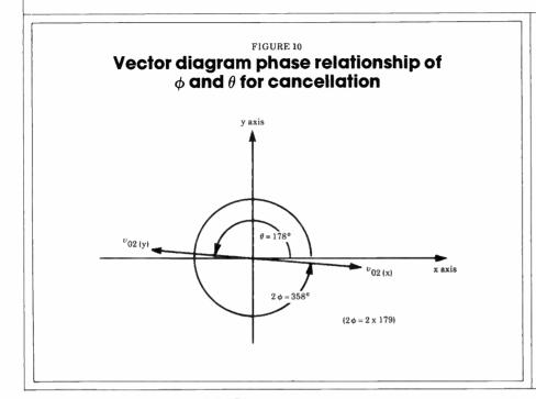
shows the improvement  $(I_{pp})$  due to push-pull versus the output inverter phase shift  $(\theta)$  for various values of  $\phi$ . As can be seen from these curves, there are many combinations of  $\phi$  and  $\theta$  which yield perfect cancellation. A vector presentation of this mechanism is shown in Figure 10. From Figure 9, it is seen that for  $\Delta=0$  dB, 20 dB of second-order reduction is possible with a phase unbalance as high as  $10^{\circ}$ .
