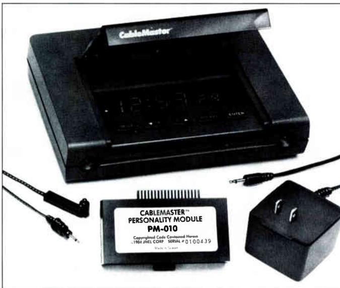
Jnel's CableMaster controls the converter with infra-red signals.
