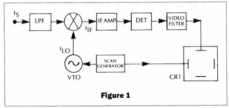
Block diagram of a swept superheterodyne spectrum analyzer. The input signal is mixed with a tuned LO frequency to produce a fixed IF which can be detected and displayed.
