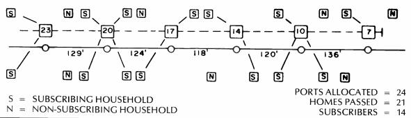
Lower tap losses. This particular example shows a loss of 1.2 dB per TGT or 4.8 dB passive loss. The traditional passive losses in Figure 1 total 8.6 dB without the terminating 7 tap! This increases the efficiency of line extender use in the system.
