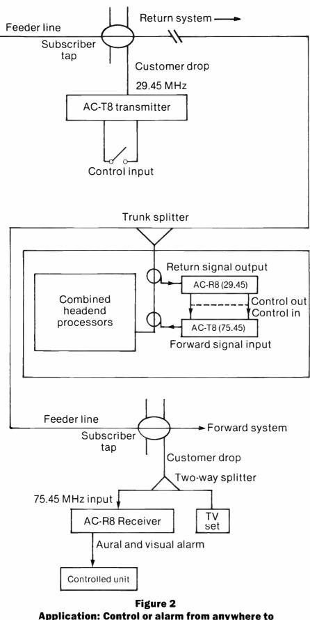
Application: Control or alarm from anywhere to anywhere in a two-way system
