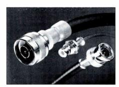
AMP Inc. introduced new cable-, paneland bulk-head-mounted 75-ohm BNC, SNB and N-Series coaxial connectors for network applications up to 2 GHz. The connectors exhibit a VSWR of less than 1.3 and RF leakage less than -55 dB (-90 dB for N-Series). Hand tools or automatic machines may be used to apply the connectors.
