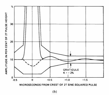
**Figure 15** Simulation of 1 MHz ringing (close-in echoes) with video resonant circuit, Q = 2.5. (a) 1 MHz circuit ringing. Unit step excitation. (b) Base of 2 T sine-squared pulse with 1-MHz ringing.
