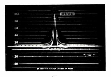
**Figure 16** Observed system response to sine-squared pulse and bar to be compared with calculated response Figure 15.(a) 2  $\,T$  sine-squared pulse. (b) 2  $\,T$  sine-squared pulse and 20- $\mu$ s white bar.
