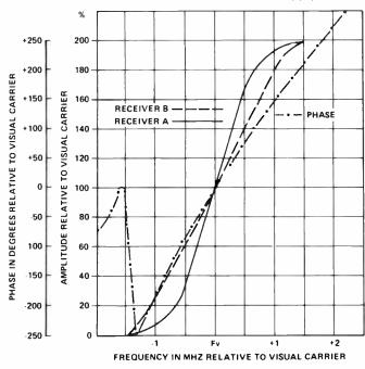
Figure 18 Attenuation and phase characteristics of representative receivers at extremes of lower sideband response.
