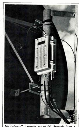
Micro-Beam™ transmits up to 60 channels from a simple tower-mounted unit—no air-conditioned buildings, extensive waveguide or expensive klystron amps
