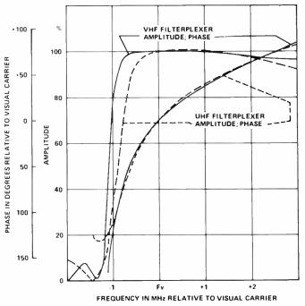
Figure 17 Attenuation and phase characteristics RCA VHF filterplexer MI-561702 and RCA UHF filterplexer MI-561543.
