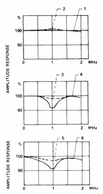
**Figure 20** System amplitude versus frequency response for various combinations of receivers and filterplexers. 1—receiver *A* and double sideband transmitter; 2—receiver *B* and double sideband transmitter; 3—receiver *A* and VHF filterplexer; 4—receiver *B* and VHF filterplexer; 5—receiver *B* and UHF filterplexer.
