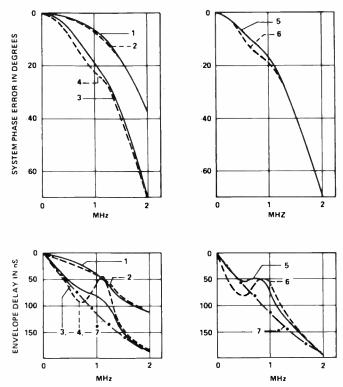
Figure 21 System phase and delay errors. Combinations of receivers and filterplexers. 1—receiver A and double sideband transmitter; 2—receiver B and double sideband transmitter; 3—receiver A and VHF filterplexer; 4—receiver B and VHF filterplexer; 5—receiver A and UHF filterplexer; 6—receiver B and UHF filterplexer; 7—appropriate transmitter delay equalization but invert slope.
