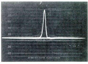
Figure 7 2  $\it{T}$  sine-squared pulse response of system. Transmitter equalizer in frequency domain with Telemet 4501 demodulator.
