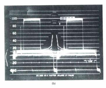
Figure 13 Sine-squared pulse and bar on Sony receiver when transmitter has been equalized for good results on R&S AMF demodulator. (a) 2 T sine-squared pulse. (b)  $20-\mu s$  white bar.
