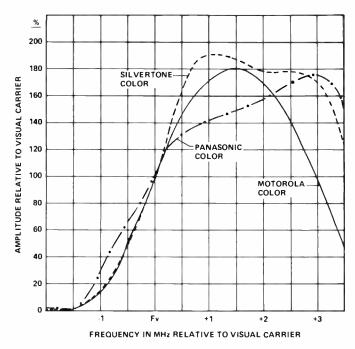
Figure 11a RF-IF attenuation characteristics of sample TV receivers1.
