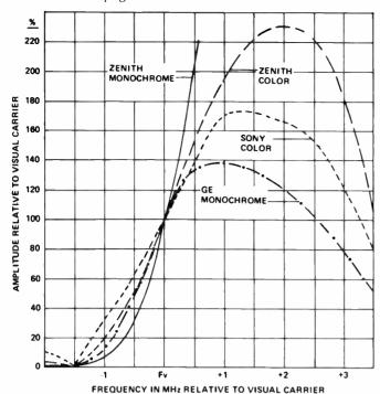
Figure 11b RF-IF attenuation characteristics of sample TV receivers1.
