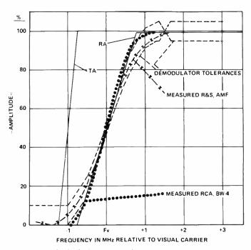
**Figure 10** Standard (idealized) RA and TA characteristics, compared to demodulator attenuation tolerances and sample measurements.
