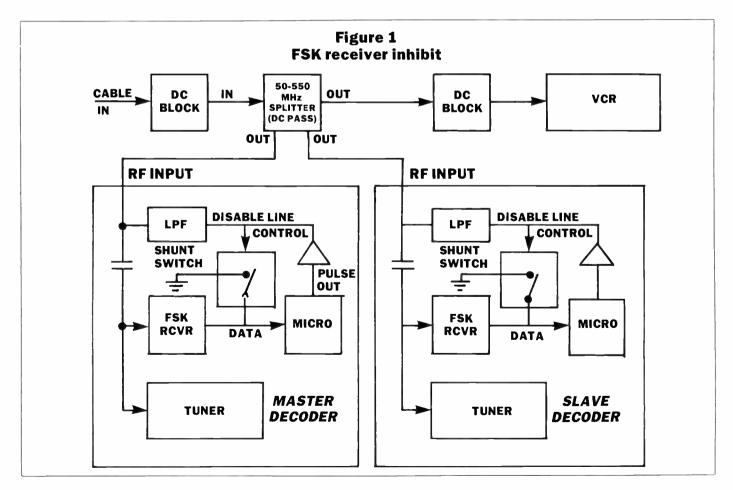
Figure 1 illustrates a functional block diagram of a master/slave configuration, the FSK inhibit approach. The master is designed to transmit a DC pulse of a certain duration to the slave that will disable the slave decoder's control data line during a deauthorize message that follows an inhibit message. (See Figure 2.) The DC pulse is put on the RF input cable of the master decoder whenever an inhibit command is received from the headend via the out-ofband standard FSK control channel.
