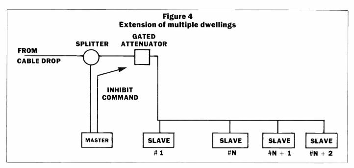
dressable cable systems using out-ofband data carrier.
