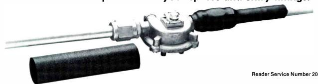
Made of radiation crosslinked polyolefin tubing, these large-expansion-ratio sleeves shrink rapidly and come with thermochromic paint and an inner adhesive lining which melts and flows to environmentally seal a connector or splice.
