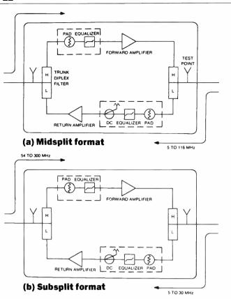
Figure 3 Typical two-way cable trunk amplifiers
