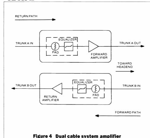
more cost effective to install two midsplit cables instead of one dual cable system. This provides 222 MHz in the return path and 464 MHz in the forward path.
