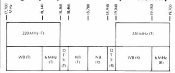
Key: DTS = Digital Termination Systems NB = 5, 10 & 20 MHz channels
