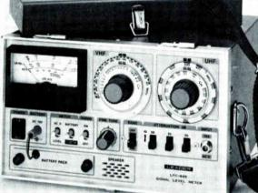
interference ratio, and image supression ratio. For CATV, you can measure the AC power on the cable.
