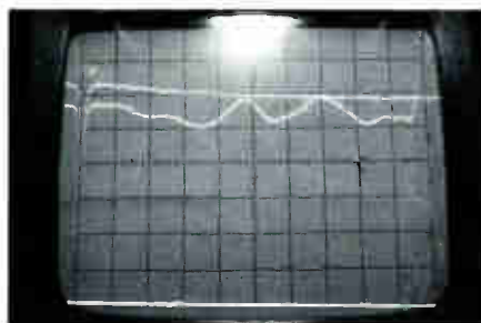
Figure 4 Standard test point showing reverse input response in high-split equipment. (1.7 dB Peak-to-Valley)
