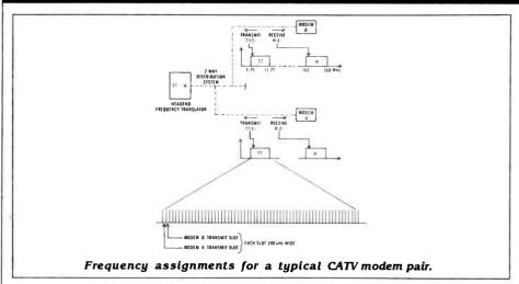
similarly connected. It is clear that there is no way in which a signal can travel directly from 'A' to 'B' using the route LE-2, TA-2, TA-3, LE-1, or vice versa. Any signal in the range 5-30 MHz will travel only toward the headend, and any signal in the range 54-300 MHz will travel only away from the headend. However, the addition of one simple device at the headend will solve this problem, and also allow great flexibility in connecting additional customers to the system.
