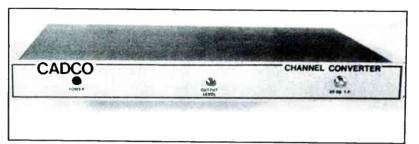
CADCO'S CHANNEL CONVERTER, Model CC 550 allows cable operators to "Cherry Pick" and rearrange single channels from a fully loaded cable system providing limited cable service to hotels, motels, hospitals, apartments, and other bulk buildings at a modest cost. This is the only processor in its price range that can accomodate a fully loaded 54 channel input. The CC 550's companion model, DATA CONVERTER DC 500 is designed for forward and reverse data transmission.
