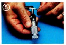
Measure the core in several places to make sure it is .143". On foil cables, measure over the foil to make sure it is .148". If out of tolerance, the connectors may not fit properly.
