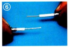
Remove a few inches of dielectric. If you find "fuzz" on the center conductor, intermittent contact may result. If the installer scrapes off the fuzz with a knife he runs the risk of damaging the copper cladding. Belden\* cable stays smooth and clean every time.
