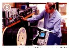
Is every reel of cable 100% sweep tested? All Belden® drop cable is (RG 59, 23 dB min.; RG 6, 26 dB min.). You don't have to accept anything less.
