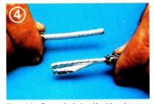
Now, strip off some jacket and braid, and expose the foil. If the aluminum/mylar shield peels off easily, it is not bonded. Duobond II\* provides a strong bond to prevent the foil from pushing back during termination.
