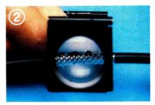
Carefully strip jacket off one inch of cable. If you ordered 67% braid, make sure 2/3 of the foil is covered by braid—not 1/2 or less.
