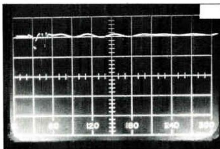
**Figure 6. Return loss of 100 ft. RG-59 terminated in 75 ohms**
