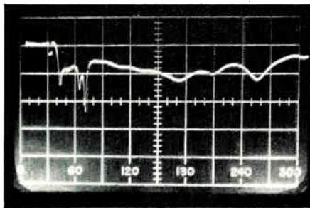
**Figure 11. Return loss of a converter tuned to channel 4/100 ft. RG-59**
