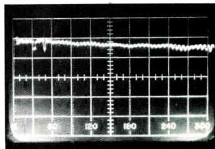
**Figure 9. Return loss of 100 ft. BAD RG-59 terminated in 75 ohms**
