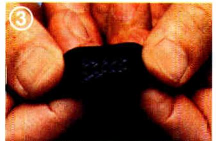
3 Check the braid impression on the underside of the removed jacket. A deep impression indicates a jacket which is too tight. This may cause difficult "F" connector installation. An extremely shallow impression indicates a jacket which is too loose.
