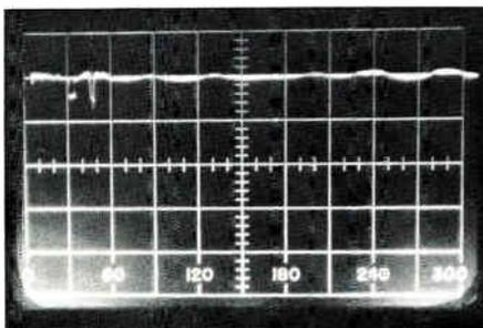
**Figure 5. Return loss of a short**
