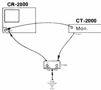
Figure 12. These connections may vary slightly, depending on the test equipment types used. The test equipment shown in Figure 12 is a return-loss bridge and standard Avantek sweep set. (Note that the auxiliary pilot input to the CR-2000 is used to prevent loss of the 50 MHz sweep sync that could occur because of the higher losses involved in the return-loss test.)
