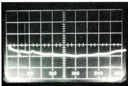
**Figure 4. Return loss of an open**
