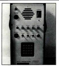
Wilk's tranceiver is a portable, battery-operated unit that will function over a wide temperature range (+50 degrees C to -20 degrees C). By connecting the unit with one coaxial cable to a test point or tap, the user can communicate with similar portables anywhere on the cable system.
