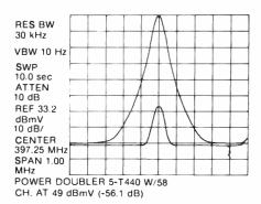
Figure 2c Unit C/CTB - power doubling At 3 dB Higher Output
