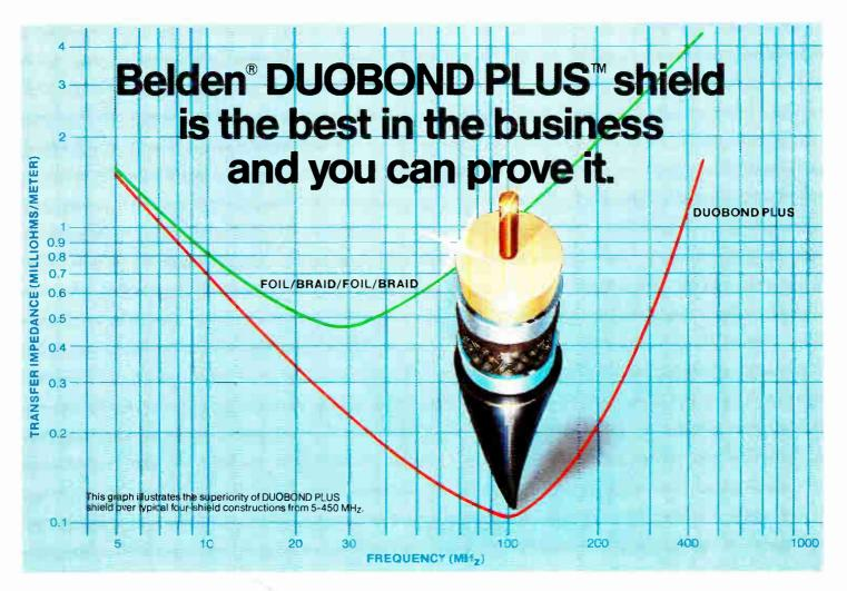
New DUOBOND PLUS drop cable shield can keep performance up and costs down in your CATV operations. Using a unique foil/braid/foil configuration, DUOBOND PLUS shield delivers greater shielding effectiveness than typical 4-shield constructions. It's also smaller in diameter, easier to terminate, lighter weight and more flexible.
