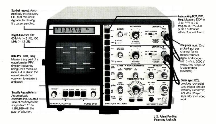
The first scope with push button digital readout. If you use general purpose oscilloscopes for trouble-shooting or testing, we can double your present productivity with the SC61 Waveform Analyzer, the first instrument to turn every conventional scope measurement into an automatic digital readout.
