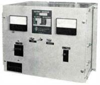
The PCP controlled ferroresonant battery charger is a real energy . typical efficiencies are over 85% with power factors over 92%. Typical Volt-Ampere conversion factors of 78% are the result of this new technology . . . compared to 50% or less with SCR & Mag-amp models. In addition to saving energy, generator size may be reduced, and due to lower BTU's air conditioing cost can be cut. PCP also manufactures power supplies
