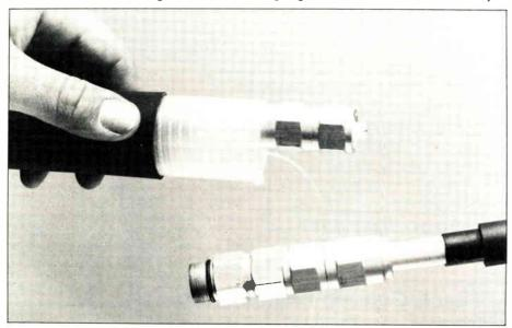
An important aspect of mechanical inspection is making sure that the heat shrink tubing has been applied properly.
