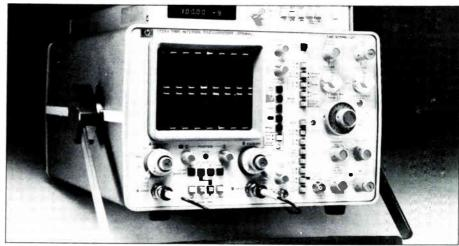
Hewlett-Packard 1726A time-interval oscilloscope
