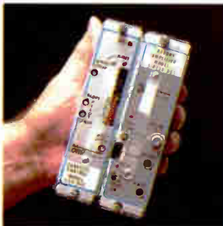
Plug the microprocessor controlled DSS and return modules into the Magna 440 main station amplifier, and you have system wide digital status monitoring.
