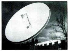
M-A/COM's 3.7-meter transportable earth station.
