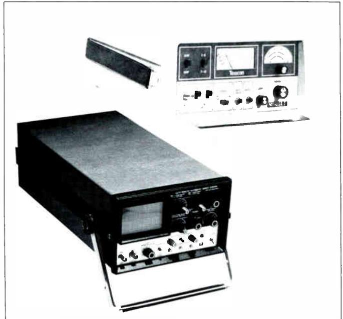
The Installer 1 signal level meter from Texscan Corporation, and the CR-2000 sweep receiver system from Avantek.
