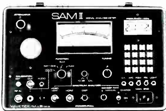
The SAM II signal level meter from Wavetek/Mid State.
