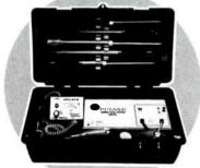
to detect the position of the fault along the conductor. The fault is located by the directional deflection of the receiver meter.
