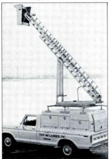
perfect workshops designed to fit either the economy-minded compact or full-size pickups. The bodies have several access points and each is protected with quality lockable hardware for added security. Each body is equipped with several removable work trays to facilitate inventory control and good organization of components. Optional shelving, interior lighting and ladder rack packages are available to maximize the utilization of the body.
