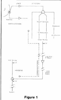
separate building is constructed to house the E.S. receivers and the necessary TV modulators. The outputs of the modulators are mixed and brought to the head-end by a coaxial cable where they are mixed with the other channels and sent into the cable system. Switching of transponders is accomplished at the remote site, and if this site isn't too far away the system works guite well.
