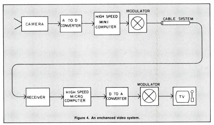
much smaller increase in bandwidth; however, about 12 MHz would still be required for each channel. Figure 4 illustrates such an enhanced digital video system. The trade-off that exists then becomes whether or not the increased picture quality is worth twice the bandwidth. When wider bandwidth transmission systems become available—for example, fiber optics—bandwidth may not be so important.
