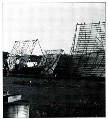
Oliver Swan at his spherical antenna farm near Bisbee, Arizona, has developed a full family of spherical antennas from 10 foot to 20 foot. Located in the 33-34 dBw contour region, even ten foot produces noise-free pictures.
