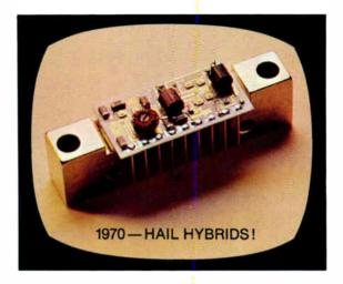
First hybrids for CATV. Elimination of interconnects provides inherent increase in reliability, ease of field repairs. Improved performance over discrete amplifiers.
