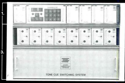
2. Expanded Basic unit provides time switching for up to eight channels with 2,552 switch functions.
