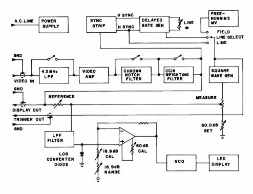
Figure 3. VNM-428 video noise meter functional block diagram.
