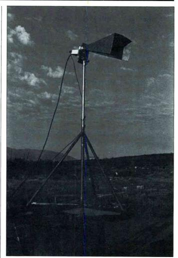
The Feed for Spherical antenna developed by Swan is approximately 23 inches long. By placing multiple feeds in front of the antenna, simultaneous reception from several satellites is possible.
