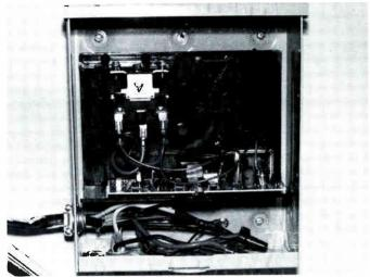
The high current controller is designed for water heater load control or other applications that require interruption of 30 amp, 240 V AC circuits.
