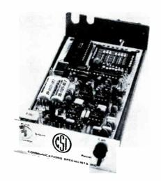
Well protected circuitry and matrix switch code settings are provided for ease of installation. Relay outputs give isolation and eliminate extra parts required for installation.
