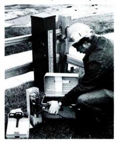
A G.E. Cablevision engineer uses the Dyna-Coupler™ to induce a tracing tone on an underground cable. This simple, clamp-like device combines the simplicity and speed of the traditional induction method with the accuracy of a direct electrical connection.
