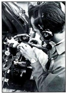
A technician prepares two lengths of fiberoptic cable for fusion splicing. The fusion splicer permits a technician to precisely align the tiny fibers and then to permanently join them in the field.
