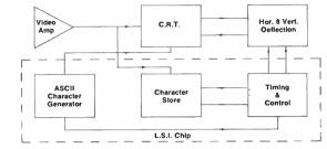
Figure 3: functional block diagram of home receiver modified to provide captioning for the hearing impaired.
