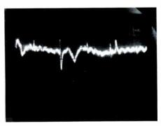
Figure 2A: analyzer response-TV set on channel 3. Note additional response at 50 MHz, and TV local oscillator.
