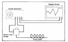
Figure 8: equipment setup for swept return loss measurement.
