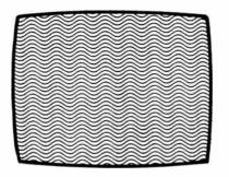
I have a Channel Commander 1 headend and have had problems with beats in the picture. The beat appears on channel 8 when channel 9 is on and disappears when I turn channel 9 off. I have seen this kind of prob-
