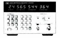
The basic model 5342A was introduced in November 1977 and offers simple keyboard control and versatility. It comes in a fieldportable package and measures frequency from 10 Hz to 18GHz with a resolution of 1 Hz on an 11-digit LED display.
