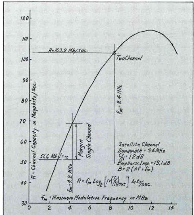
Figure 3. Information rate vs. modulation frequency
