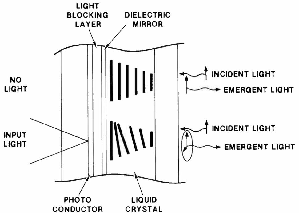
Figure 1: Functional diagram of the hybrid field effect liquid crystal light valve.
