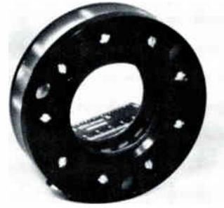
The liquid crystal light valve is a new electro-optic television projector display device. It uses liquid crystal chemicals and thin film, solid state electronics to permit the projection of television images onto a large screen.
