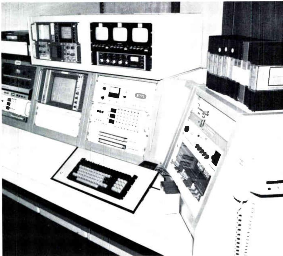
*This three-channel airing facility console incorporates a color monitor, vectorscope, wave form monitor and time base correctors.*
