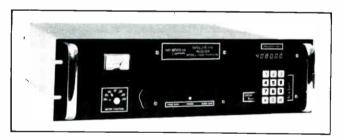
Microdyne digitally tuned receiver permits rapid channel selection and excellent frequency stability.
