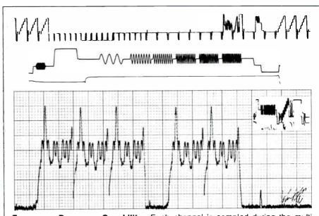
Frequency Response Capability-Each channel is sampled during the multiburst portion of the vertical interval. All bursts including the upper and lower sideband are shown.
