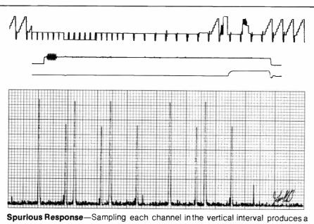
display without frequency components other than the picture and sound carriers. 30 kHz I.F. bandwidth was used. Vertical resolution is 20 dB per major block.
