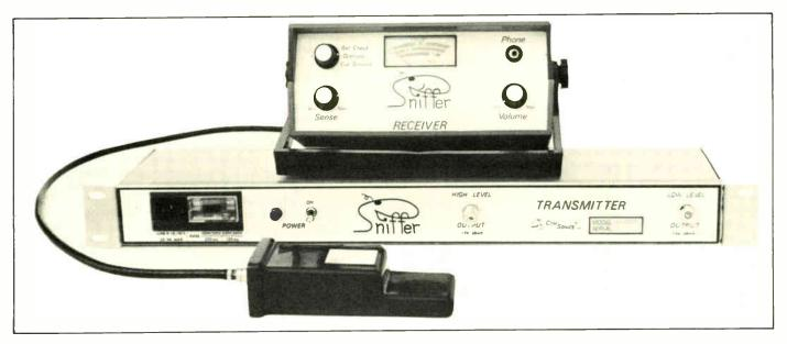
pinpointing and cleaning up shielding flaws is the purpose of a leakage detection system. Rapid leak location can be obtained only by equipment designed for near and far field detection, AND near field isolation.
