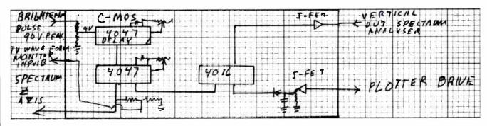
Schematic of sampling pulse generator.
