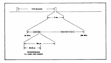
Figure 2 Timing Diagram—Simultaneous Sweep
