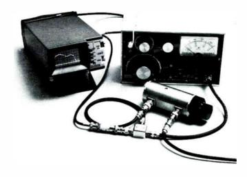
Figure 8 Convenient Portable Simultaneous Sweep Receiver Using the New Tektronix 214 Portable Storage Scope.
