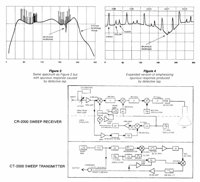
**Figure 5** Simplified Block Diagrams of the Avantek Sweep System
