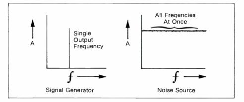
Figure 2—Difference Between Signal Generator and Noise Source.
