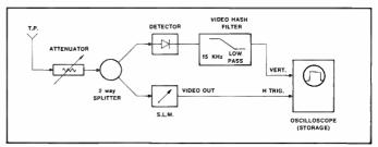
Figure 3 Connections of Test Equipment
