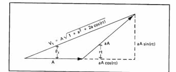
Figure 2. Discriminator Output Phasor Diagram
