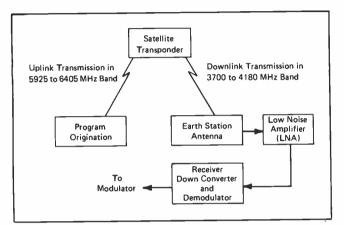
Figure 1. Satellite-Earth Station System, Block Diagram
