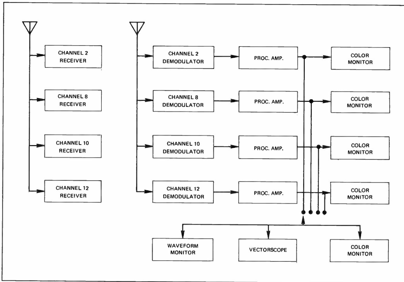
Figure 4. Equipment at Receiving Site
