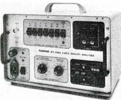
the nature and severity of the fault. It will detect opens, shorts, frays and crimped cable as well as faults in splitters and can also be used to detect faults and accurately find the length of cable while still on the reel. It will "look beyond" discontinuities on a cable, or beyond several splitters or other in-line devices, to find faults further along the cable run. Unauthorized connections to CATV drops can be detected even when isolated with a splitter.
