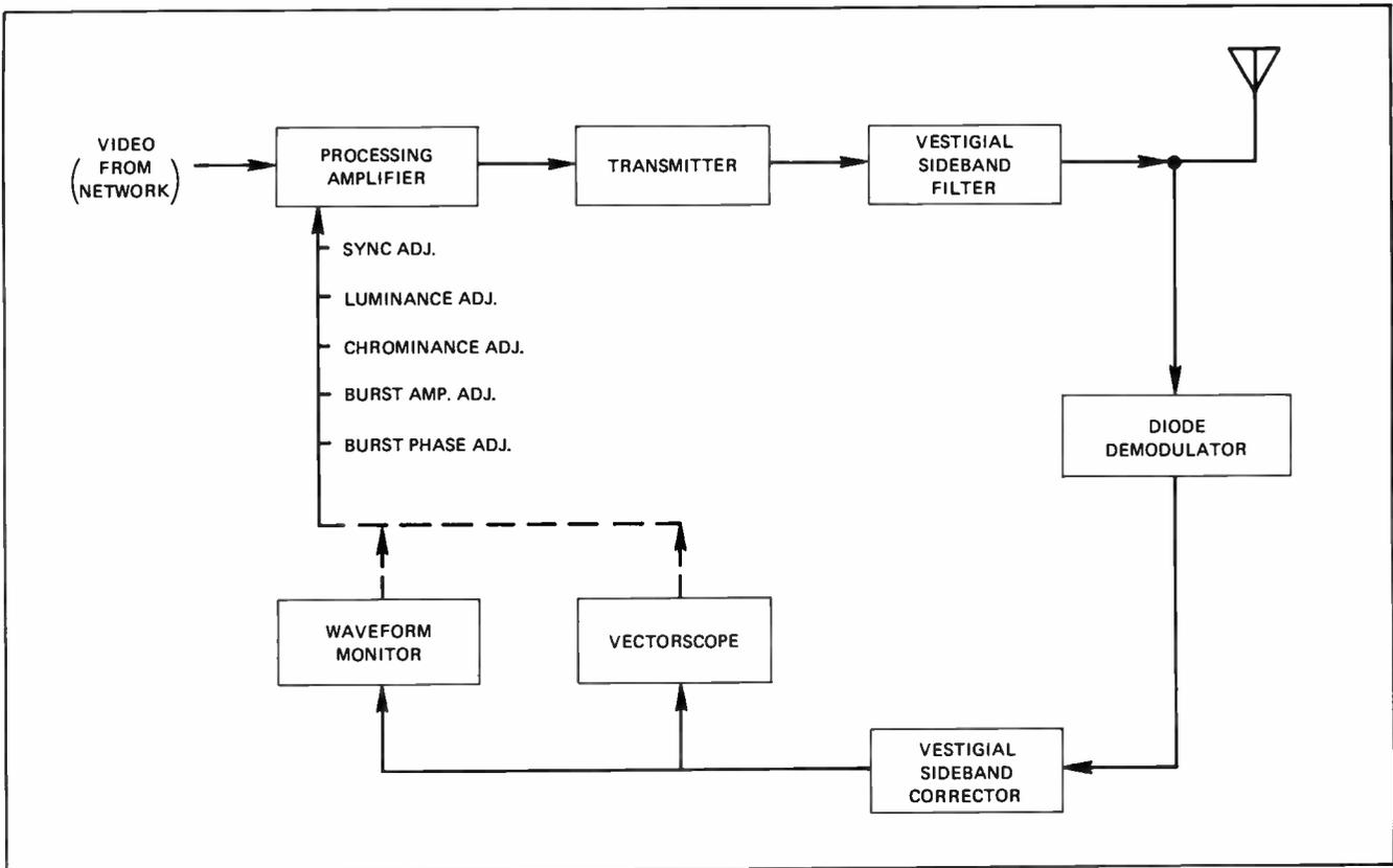
Figure 3. Equipment at Transmitters
