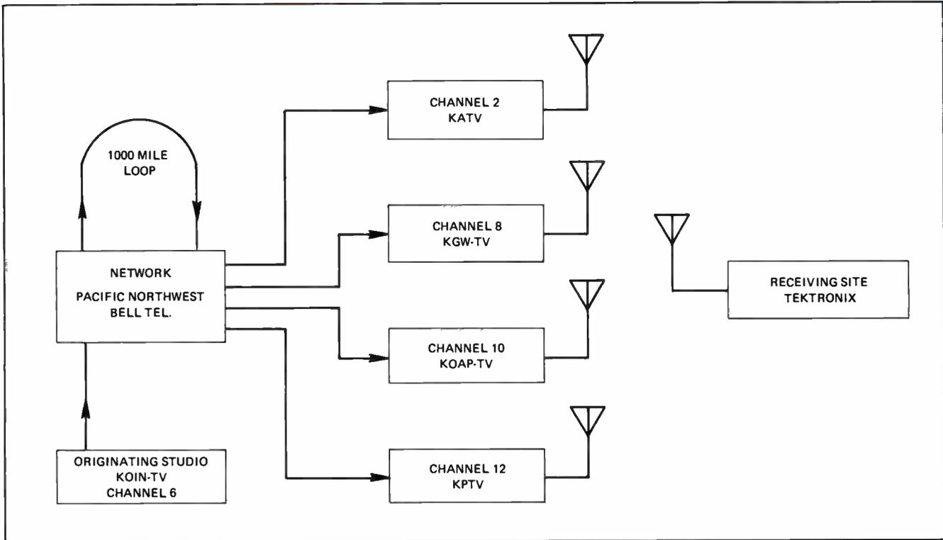
Figure 2. System Diagram—VIR Subjective Field-test
