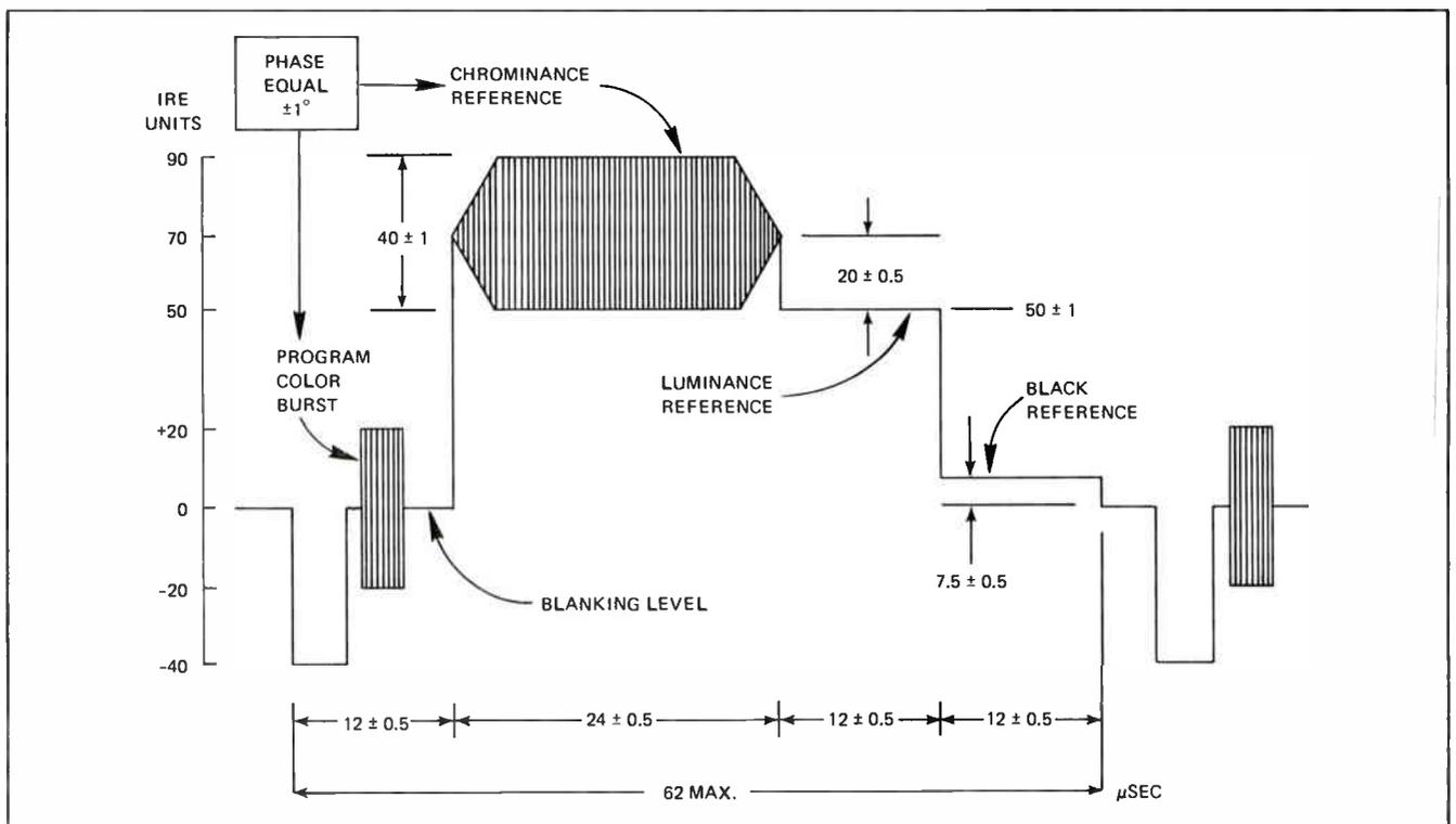
Figure 1. VIR Signal—Inserted on Line 19, Both Fields
