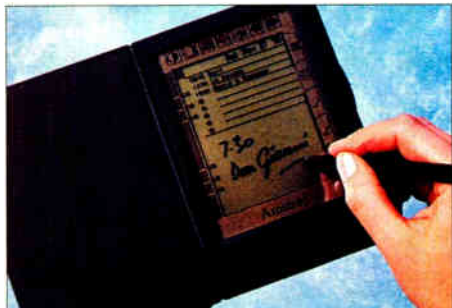
The Pen Pad weighs less than a pound and is solely pen-operated, with no external (or emulated) keyboard option.
