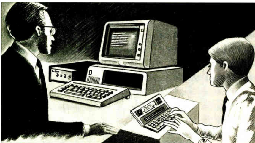
This deaf user's PC is connected to a telephone via an Ultratec Intel-Modem Baudot/ASCII modem. The user is sending and receiving messages to and from someone at a remote site who is using a telecommunications device for deaf people (right).
