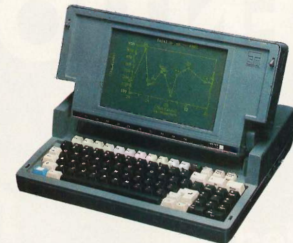
The STM LapTop connects to the LapMate expansion unit.
