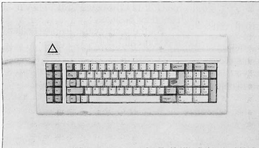
Photo 1: The Model D's 83-key QWERTY keyboard.
