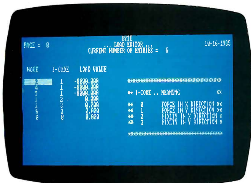
Photo 1c: A screen image of the load editor with data for the truss shown in figure B.
