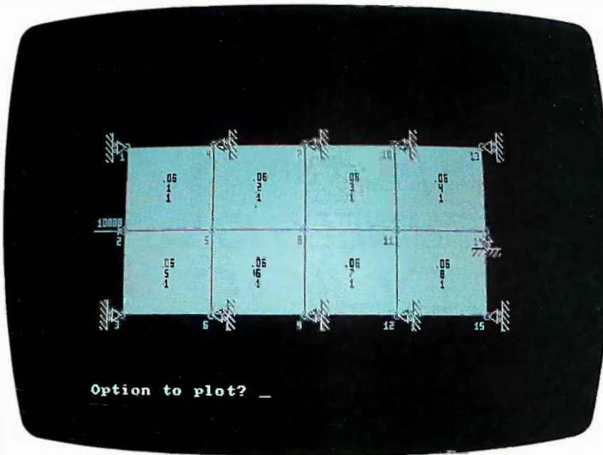
Photo 1: Plot of the stiffened panel with a 10,000-pound load on the central stiffener, drawn by the SAFEPL0T.EXE program.
