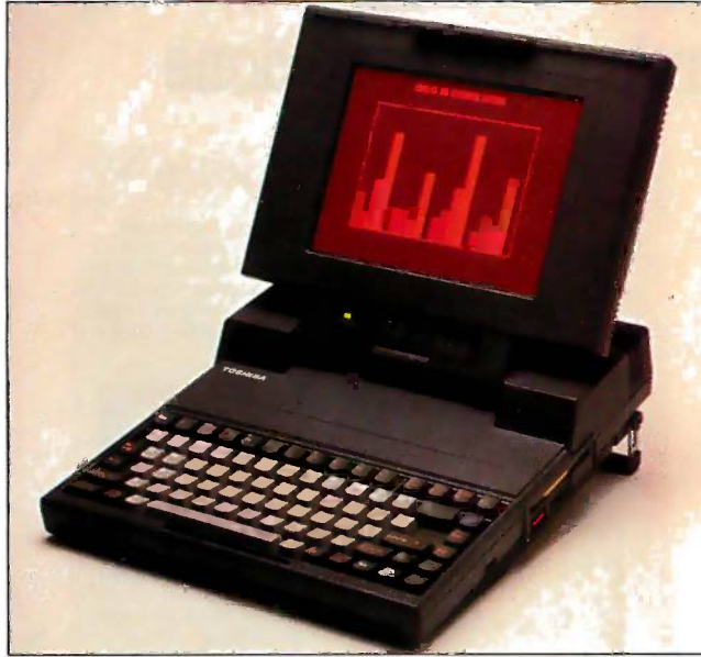
Toshiba's T3100, a portable with a gas-plasma display and internal hard disk drive.
