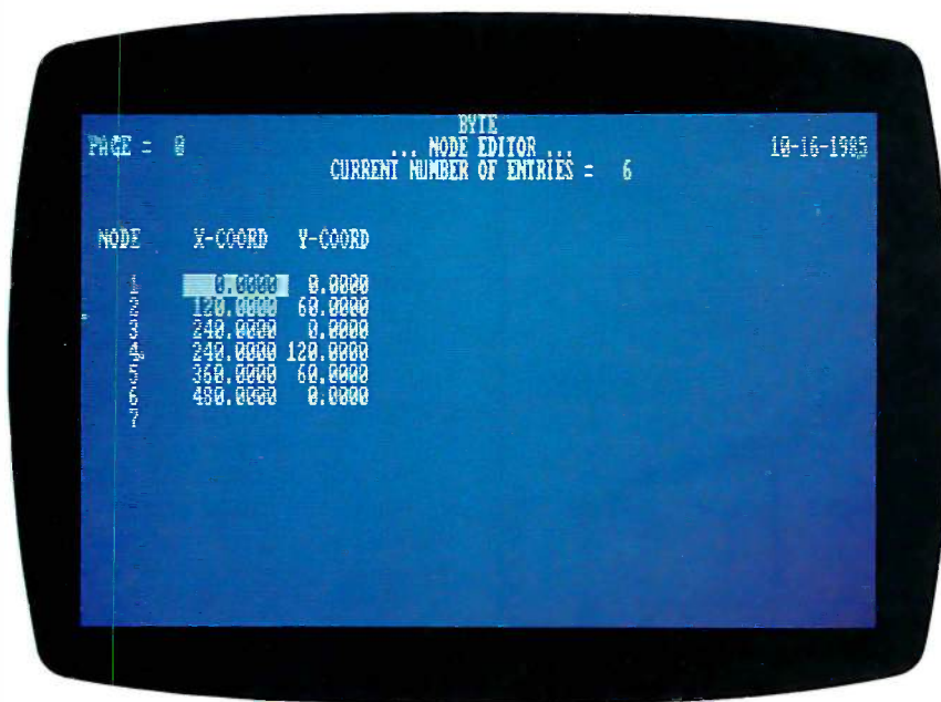
Photo 1a: Data entry and modification is done through the node, element, and load screen editors. Pictured is a screen image of the node editor.
