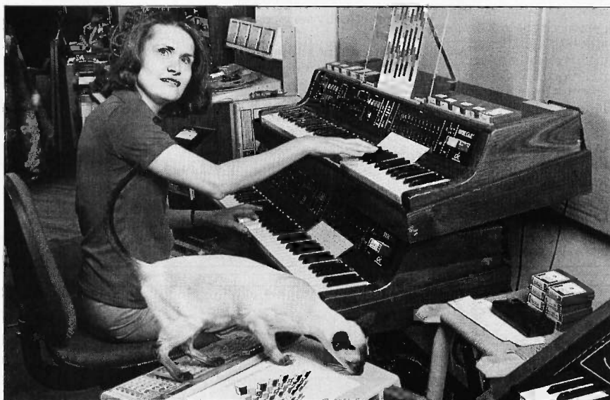
Photo 3: Wendy Carlos, in her studio, illustrating the Synergy, Hal Alles's harmonic-synthesis synthesizer. (Photo by Vernon L. Smith.)
