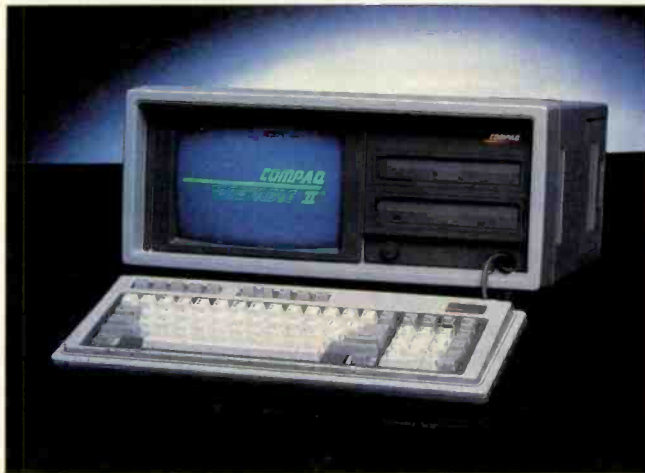
The Compaq Portable II runs on an 80286 processor.
