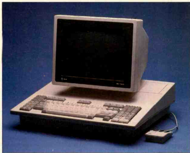
Photo 1: The AT&T UNIX PC showing tilt-and-swivel display, keyboard (not extended; disk drives are covered by the keyboard in this photo), and the three-button mouse.
