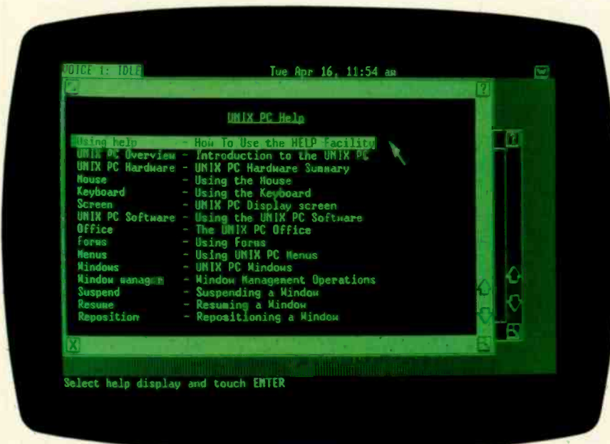
Photo 2: The AT&T UNIX PC display screen showing two overlapping windows. Status of communications lines is shown at the top left, followed by the internal clock date-and-time display.
