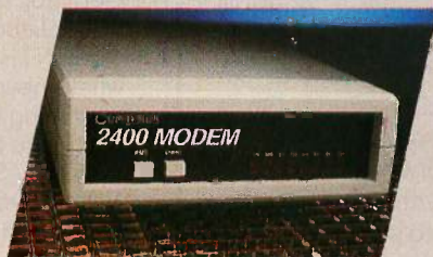
2400 Modem - A Hayes™ compatible 2400 bps modem with intelligent features and built-in diagnostics. MNP error control is available on the 2400 EP Modem.
