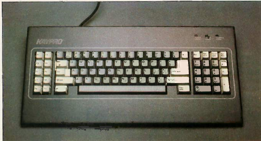
Photo 1: The Kaypro 286i keyboard uses the IBM PC AT layout.
