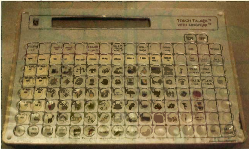
Photo B: The Touch Talker keyboard. Note the keyguard to prevent those with motor-coordination difficulties from activating the wrong key. This device also requires a pressure of 4½ ounces to initiate a keystroke, enabling those who have problems controlling fine movements to select only the key they really want. (Photo by Robin Schwartzmiller.)
