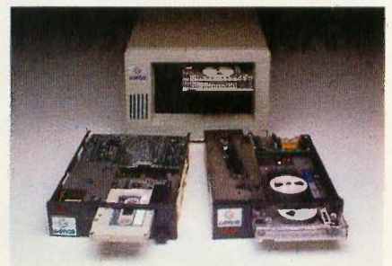
The IBM®-compatible Genoa Galaxies are available as internal or external versions of 1/4" streaming tape or cassette models. (External cassette not shown.)
