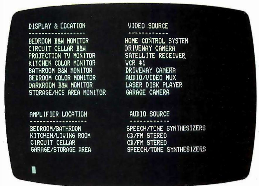
Photo 3: Using the BCC-52 and a video-display controller, a display of the AVMUX's configuration by location and source is easier to read than LEDs.
