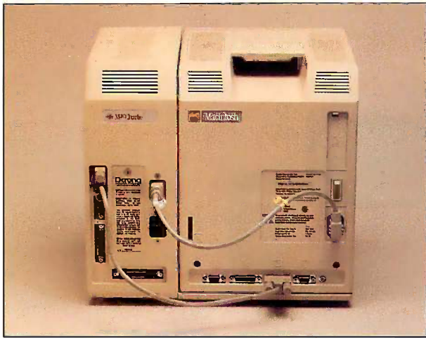
The rear of the Macintosh/MacCharlie systems. Note that the Mac gets its power from the MacCharlie unit. The Mac printer port is dedicated to communicating with MacCharlie.
