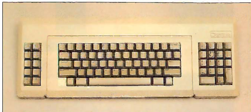
Photo 2: The MacCharlie function keys and numeric keypad attach to the Macintosh keyboard.
