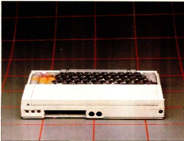
The rear panel reveals (among other things) a speaker jack, an expansion bus, and an RS-232C port.
