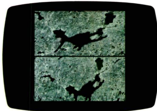
Photo 2c: Upper portion is original data, lower portion has been rectified to a base map.
