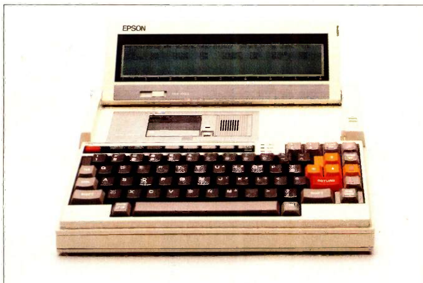
Photo 2: The display of the Epson PX-8. Under certain lighting conditions this 80-character by 8-line display can be difficult to read.
