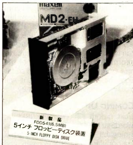
Photo 1: The 6.5-megabyte floppy-disk drive from Hitachi.
