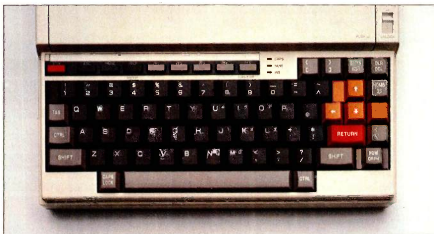
Photo 3: The keyboard of the Epson PX-8. In this picture the display is folded down over the microcassette drive. Note the second Control key to the right of the space bar and the caps-lock, num-lock, and insert-mode indicators above the zero key.
