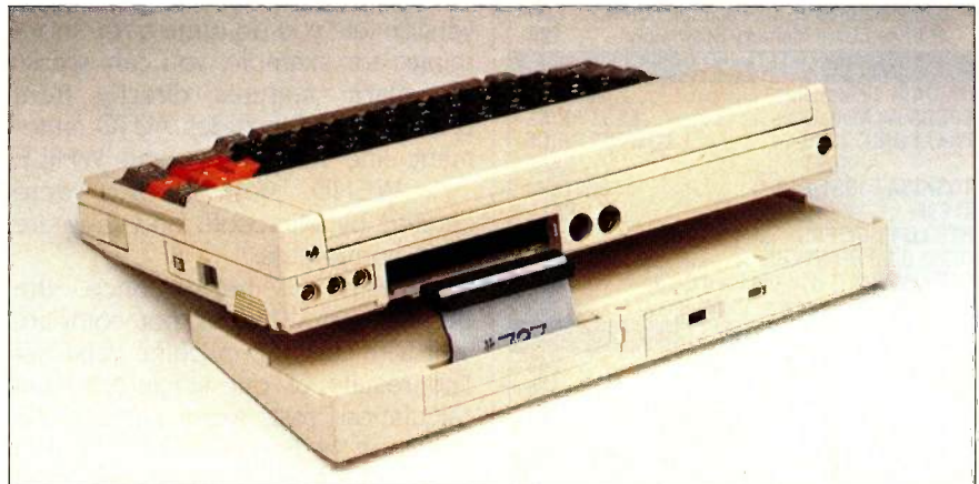
Photo 4: The optional memory-expansion module for the Epson PX-8, shown ready to attach to the bottom of the computer.
