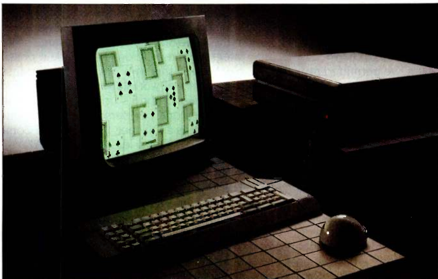
Photo 1: The Whitchapel Computer Works MG-1 uses the National Semiconductor 32016 32-bit virtual-memory processor chip.
