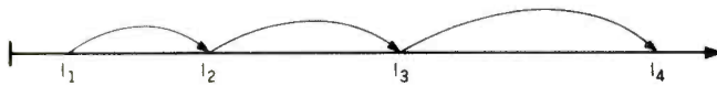
Figure 1: Schematic diagram of mapping in a linear congruential generator (LCG). Each successive term in the series is larger than the preceding. This series does not imitate a random series, but it is the first step in that direction. See figure 2.
