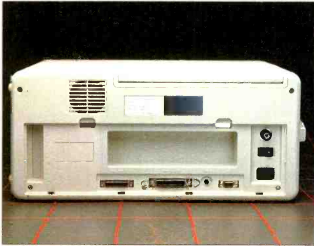
The rear panel of the Panasonic Sr. Partner. Along the bottom are a serial connector, a parallel printer connector, the brightness control for the display, and an RGB color monitor connector. The power switch is on the right. On the left is a removable plate hiding an expansion slot.
