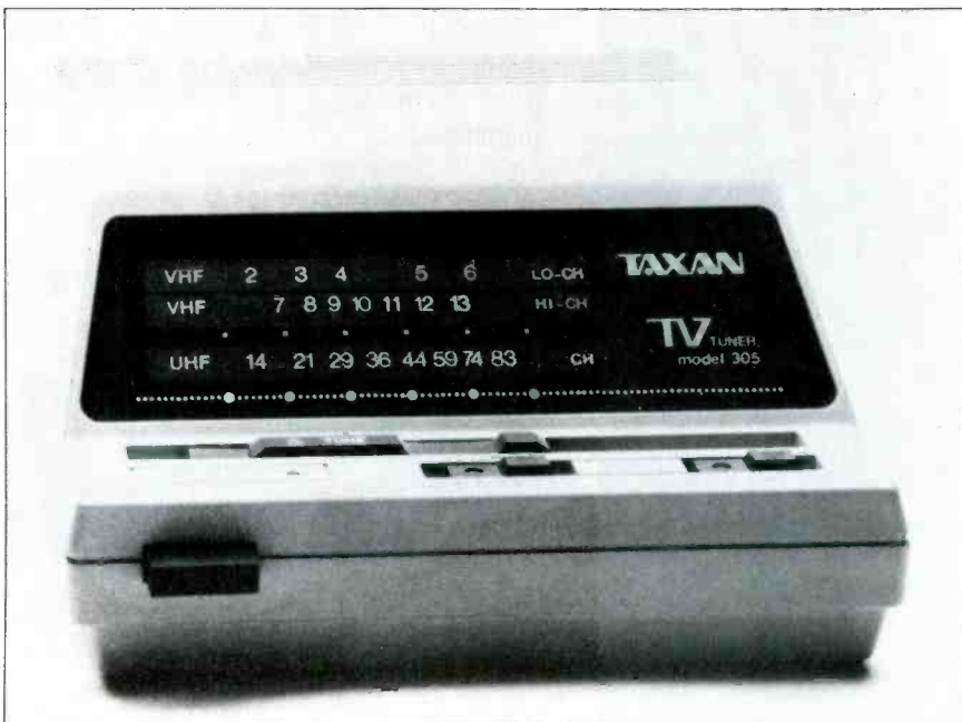
Photo 1: Taxan's Model 305 tuner converts a color monitor into a television.
