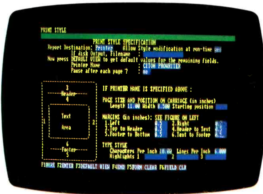
Photo 4: DataEase print-style-selection screen for entering custom printer, page, and other settings for a report. These may be modified prior to printing the report.
