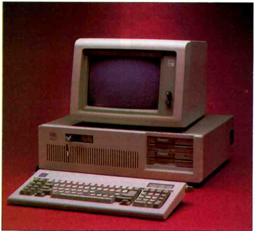
Photo 1: The IBM PC AT with a 20-megabyte hard-disk drive. This unit is equipped with an IBM monochrome monitor and a second, 360K-byte floppy-disk drive. Note the switch lock on the front panel.
