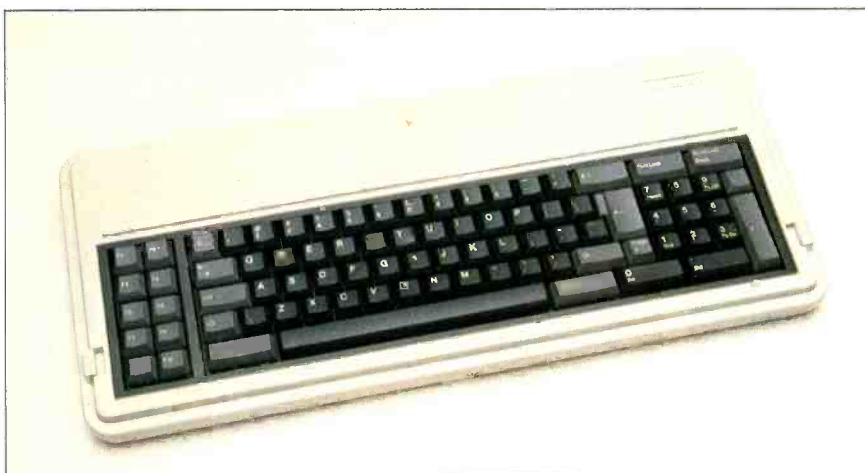
Photo 3: The keyboard of the Panasonic Sr. Partner. Note the oversize Return and Shift keys.
