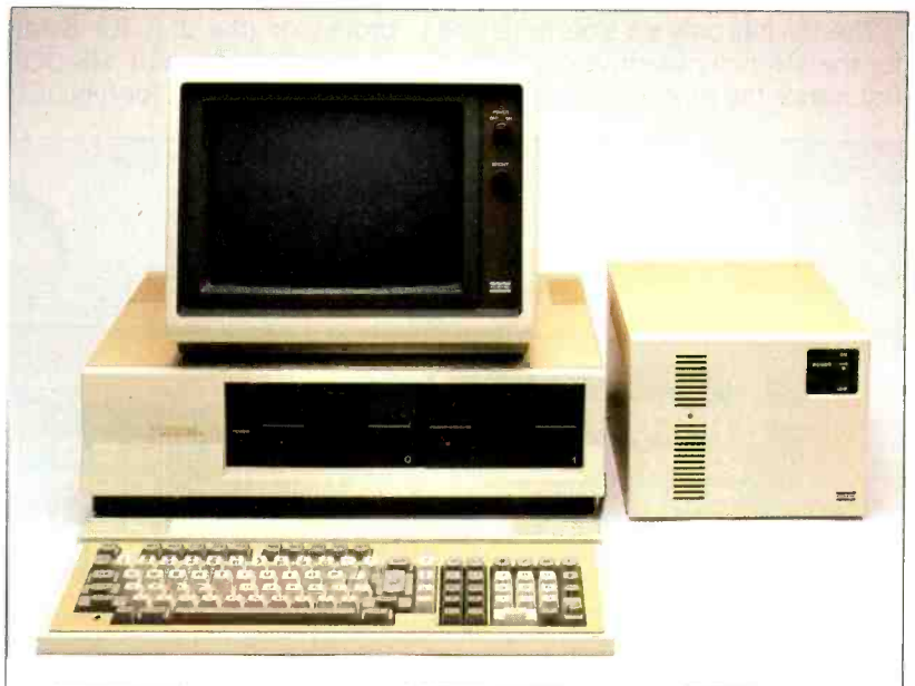
Photo 1: The Fujitsu Micro 16s and an optional 13-megabyte 5¼-inch hard-disk drive.
