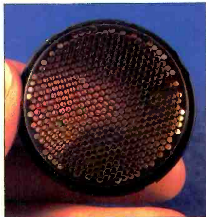
Photo 2: A close-up of the Polaroid ultrasonic transducer.
