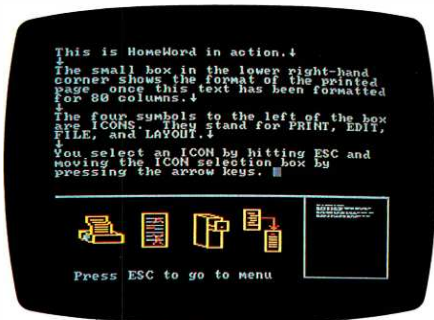
Photo 4: HomeWord, an easy-to-use word processor for the IBM PCjr, features a text-edit area; icons for selecting print, edit, file, and layout functions; and a box containing a graphic representation of the current page's format.
