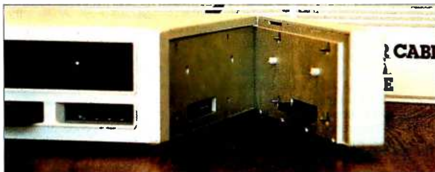
Photo 5: Some options, such as the parallel-printer adapter shown here, attach to the bus connector on the right-hand side of the PCjr.
