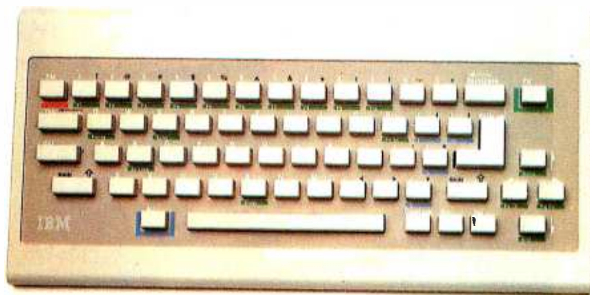
Photo 2: The infamous PCjr keyboard features widely spaced keys and legends that are hard to read from a normal typing angle.
