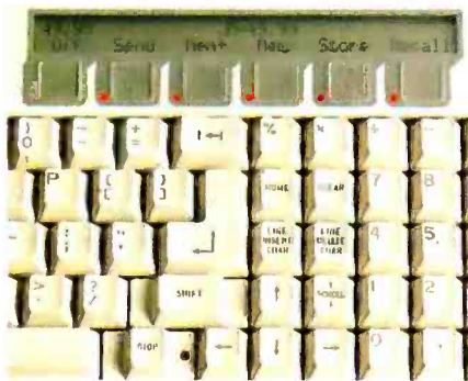
The unique MicroScreen™ serves as a calendar, clock, a built-in calculator, and a labelling device for special touch-sensitive keys.
