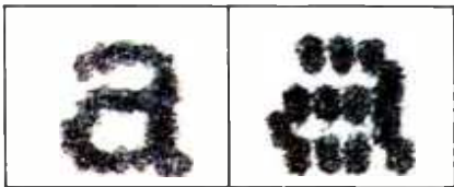
Our exclusive 18-pin print head is graphically sharper than a 9-pin printer, as this unretouched photo shows.
